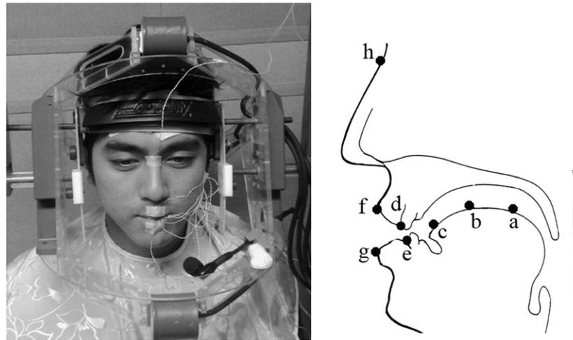
**Fig. 1.** The experimental setting of the EMA system and locations of sensors: (a) the tongue dorsum; (b) the tongue midsection; (c) the tongue tip; (d–e) the maxillary (upper) and mandibular (lower) central incisors; (f–g) the upper and lower lips; and (h) the nose bridge.
